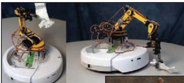
Top: iRobot Create modified with robotic arm and end effector that can pick up paper
