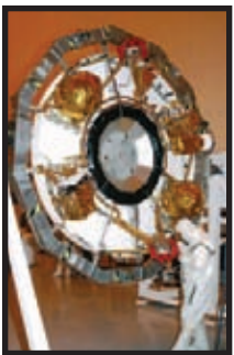
Left: Bottom cruise ring for Mars rovers (black inner ring contains the low and high-gain antennas)
