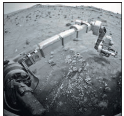
Mars rover Spirit's robotic arm with 5 degrees of freedom
