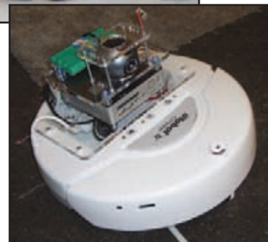
Top: iRobot Create modified with robotic arm and end effector that can pick up paper
